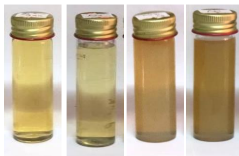
Fig. (1) Photographs of the optimum samples prepared after 9 minutes reduction time with different concentrations of Ag colloids (left to right: 2 \times 10^{-3} , 3 \times 10^{-3} , 4 \times 10^{-3} and 5 \times 10^{-3} mol/L)
